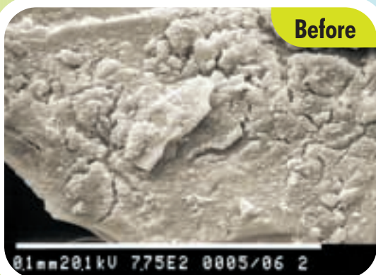
A typical scanning electron microscope picture of a sand grain before application of AQUA-ZORB, showing the hydrophobic coating
